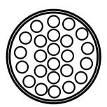
Jacketed pneumatic tube, high density polyethylene.
